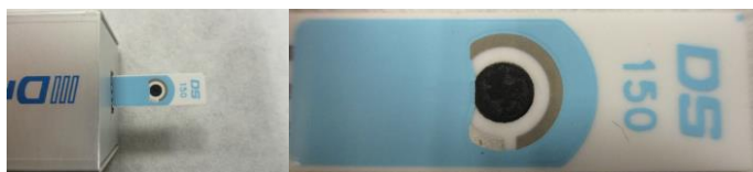
Figure 36: photography of modified DropSense 150 screen-printed electrodes.
