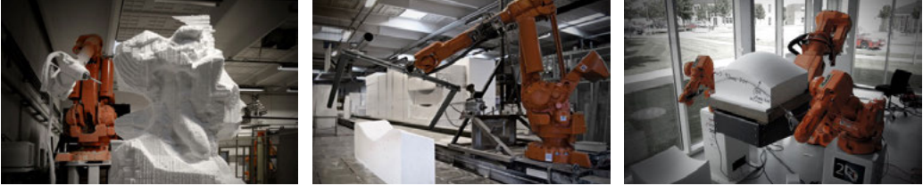
Figure 1. Different cutting techniques: CNC-milling, hot wire cutting, and hot-blade cutting.
