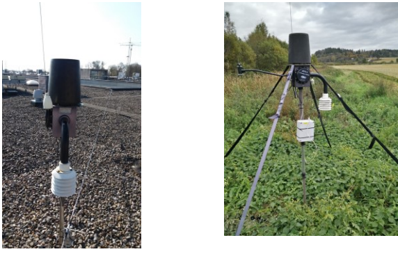
Fig. 4. Automatic Weather Station with RF1 module inside
