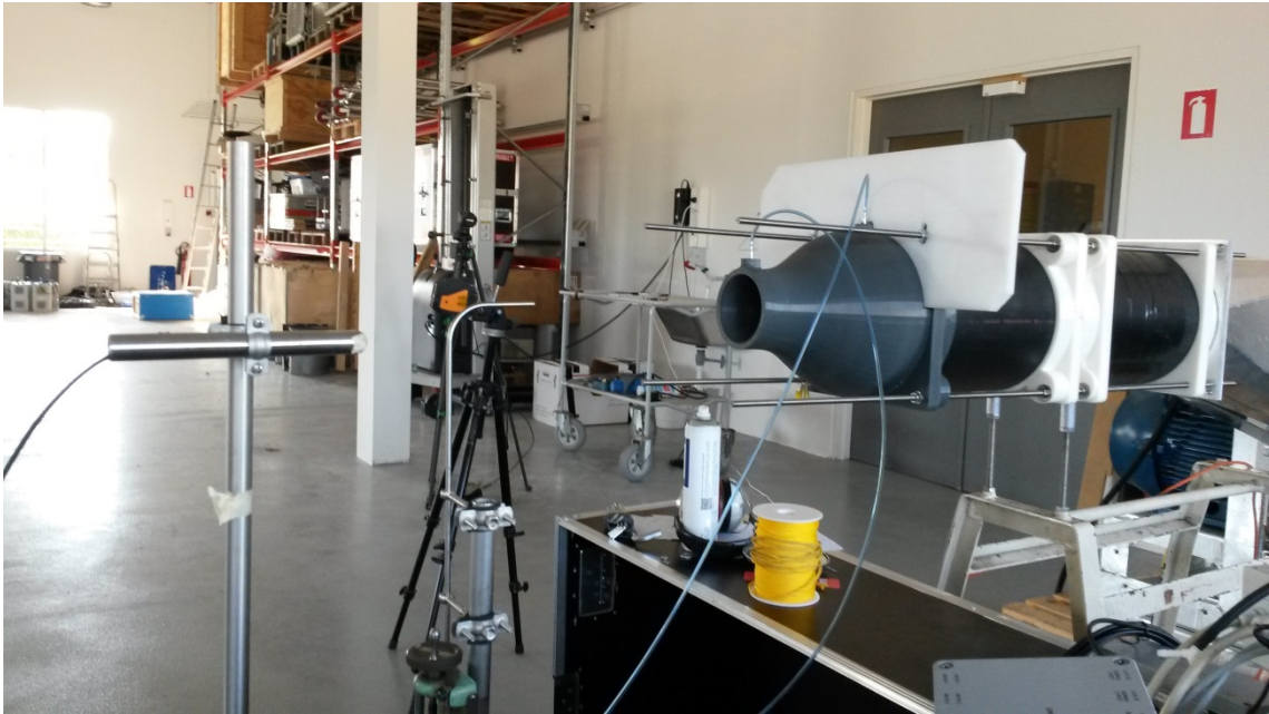
Figure 99 Prandtl tube placing after the blower
