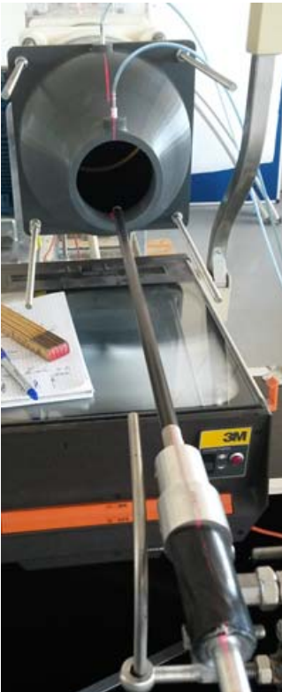
Figure 90. Pitot and prandtl not aligned
