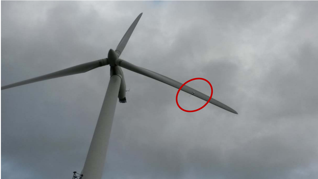
Figure 141. Photograph of the turbine with the encircled pitot measurement device
