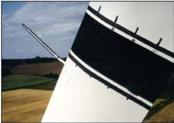
Figure 1 Pitot sensor on 100 kW wind turbine blade
