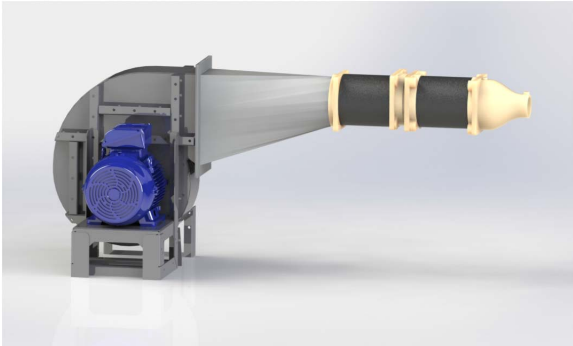
Figure 77 Rendered view of the fan, housing and motor with the in-house built adapter
