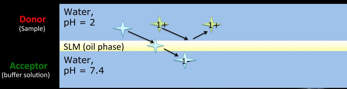
EXPERIMENT ONGOING: By choosing a pH above (below) the pK<sub>a</sub> of the acid (base) in the acceptor buffer, the analyte is trapped. While continuing to replenish the donor, both separation and enrichment of the target analyte is possible.
