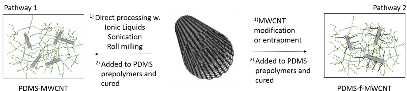
Figure 1: Dispersing MWCNT effectively in PDMS by Pathway 1 - Direct processing or Pathway 2 - Modification or entrapment and subsequent crosslinking.
