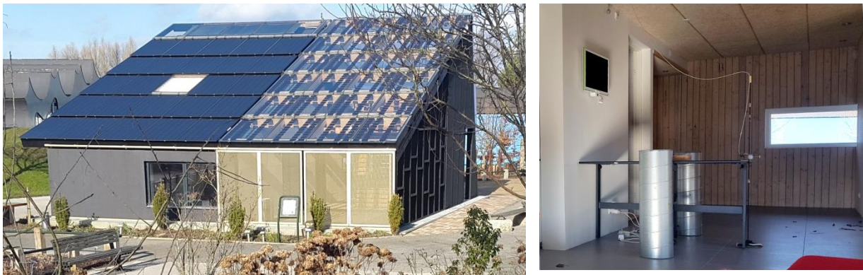
Figure 1. Outside view of the house from South-East (left), and inside view of the experimental setup with the thermal dummies (right).
