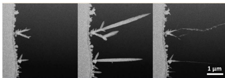
Figure 3. Dendrite growth and collapse during voltage cycle from lead nitride solution in a liquid cell (White et al., ACS Nano (2012)). 22
