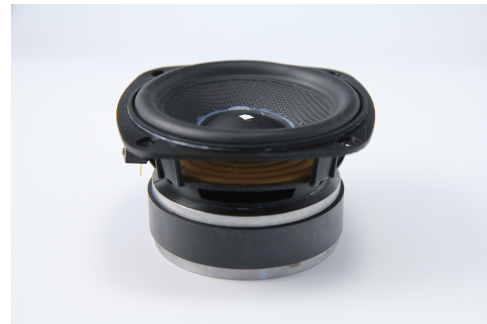
(b) Custom made driver with R_E = 1.7\Omega using a rectangular winding layout.
