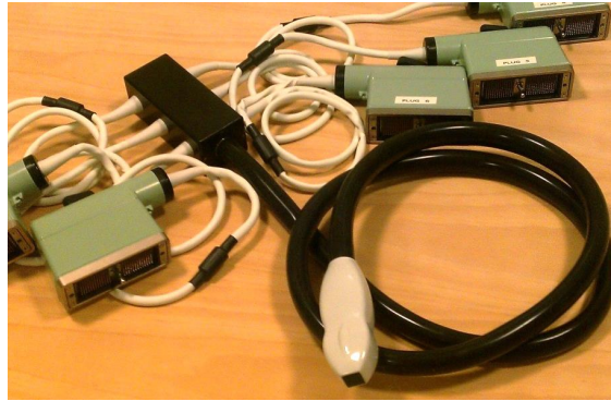
Figure 4.2: The 32 \times 32 Vernon phased matrix array with all its cables and connectors.
