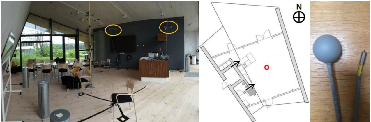
Figure 3. Panoramic view of the interior (left), the measurement location (middle) and the globe and air temperature sensors (right)
