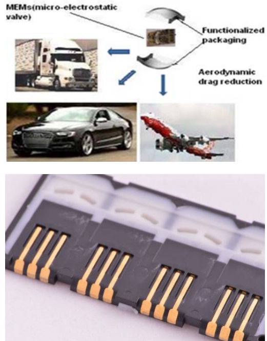
Figure 2: Micro-actuator for fluid flow control and drag reduction (top); overmoulded and plated functional micro packaging (bottom).
