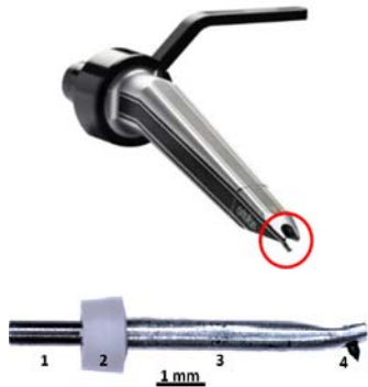
Figure 5: Cartridge (top); multi-material micro sensing actuator produced by micro insert moulding: (1) magnet, (2) suspension ring, (3) cantilever tube, (4) diamond tip.
