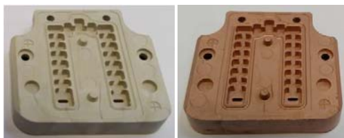
Figure 6: Injection moulded diplexer (left); plated diplexer (right).
