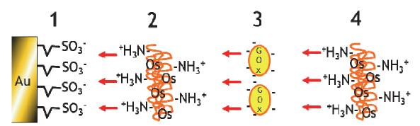
Figure 1. Schematic of self-assembled Layer-by-layer Glucose microsensor
