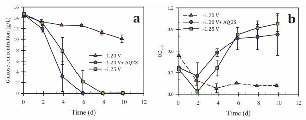
**Figure 1**. Glucose concentration (a) and growth (b) in bioelectrochemical cathodes inoculated with *C. glutamicum* in the presence or absence of 0.1 mM AQ2S.
