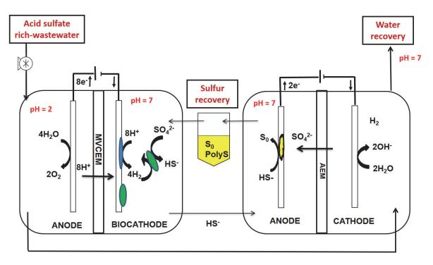
**Figure 1.** Proposed integrated autotrophic bio-electrochemical process for treatment of sulfate-rich wastewater.
