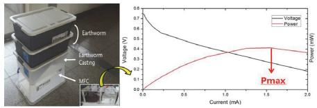
Figure 5. Vermicompost MFC system and its output characteristic
