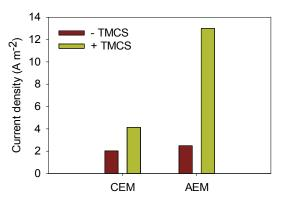
**Figure 4** Produced current densities (A  $m^{-2}$ ) for both AEM and CEM, with and without TMCS module. Transport of  $CO_2$  and  $NH_3$  via the TMCS module results in a higher current at the same applied voltage.
