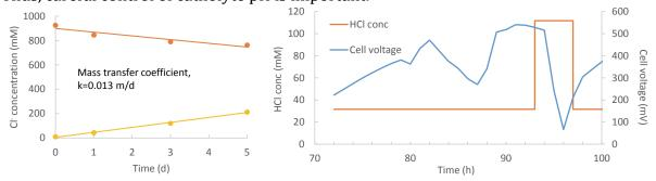
Fig. 1. (Left) Diffusion of Cl- through the AEM. (Right) HCl concentration in catholyte and cell voltage over a  $100~\Omega$  resistor.
