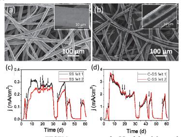
**Figure 1**: Representative FESEM images of SS felt (a) and C-SS felt (b); bioelectrocatalytic current generation for SS felt (c) and C-SS felt (d).
