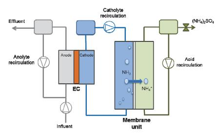
**Figure 1.** Schematic representation of the experimental setup. EC= Electrochemical Cell.
