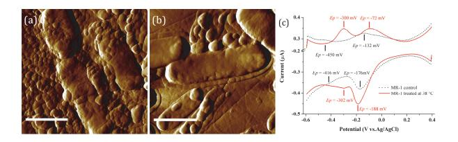
**Figure 1** Atomic force microscopy shows more EPS surrounding the MR-1 cells in control groups treated 30 °C (a), comparing to those treated at 38 °C (b). Scale bar: 2  $\mu$ m. Voltametric analysis of MR-1 treated at 30 °C (dotted line) and 38 °C (solid line) (c).
