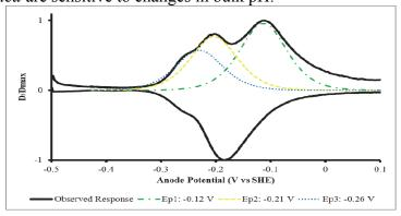
**Figure 1.** Observed derivative CV (1mV sec<sup>-1</sup>) response (black line) of *T. ferriacetica* at pH = 5.2 shown with Nernst-Monod derivative fits for:  $E_{p1} = -0.12$  V vs SHE (green hashed line),  $E_{p2} = -0.21$  V vs SHE (yellow hashed line), and  $E_{p3} = -0.26$  V vs SHE (blue dotted line).
