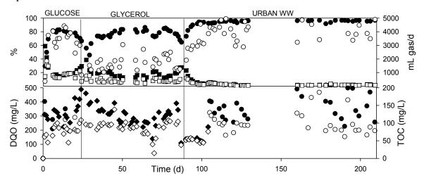
Experimental profiles for the last 8 months of continuous operation of the pilot-scale MEC: UP  $\bullet$  (%H<sub>2</sub>),  $\circ$  (mL H<sub>2</sub>/d),  $\blacksquare$  (% methane),  $\square$  (mL methane/d) and DOWN:  $\blacktriangledown$  (TOC inlet),  $\nabla$  (TOC out),  $\spadesuit$  (COD inlet),  $\diamondsuit$  (COD out).
