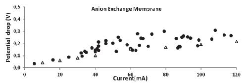
**Figure 1:** AEM membrane potential drop as function of current in biotic operation (black circles) and abiotic galvanostatic tests (white triangles)
