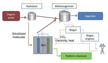
treatment facilities to promote the emergence of environmental biorefineries where oxidation of waste would be Figure 1: Mainstream scenario studied for the coupling of a BES coupled to the production of to an existing organic waste treatment facility.
