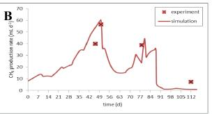
Figure 7 – Experimental and simulated evolution of MFC current (A) and CH<sub>4</sub> (B) generation over time.
