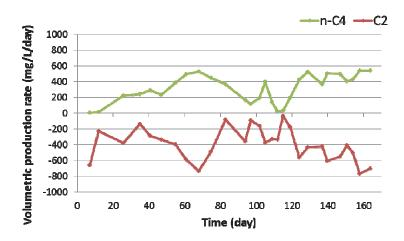
**Figure 2**: Volumetric production rate of MES cell applied with 9.3 A/m², showing n-butyrate (n-C4) production and acetate (C2) consumption during the experiment.
