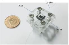
Fig. 1. Miniature single chamber MFC used in this work
