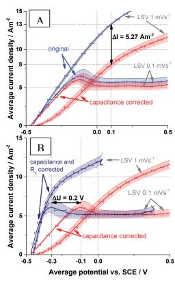
**Fig. 1**: Triplicate curves obtained in same system: activated carbon cloth (CTex13) characterized with *G. sulfurreducens* in a continuous system (HRT=24h)
