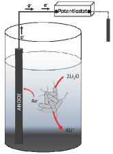
because we are committed to increase recovery and reduce the process time for competitive and manageable levels required at industrial scale, we intend to accelerate the kinetics of lithium electrobioleaching using a bioelectrochemical system. To this aim, batch experiments were carried out to evaluate the feasibility of using insoluble electrodes to stimulate mediated microbial lithium catalysis.
