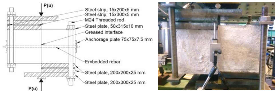
Fig. 2 Push-off test setup for shear loading (left) and a specimen during test (right)
