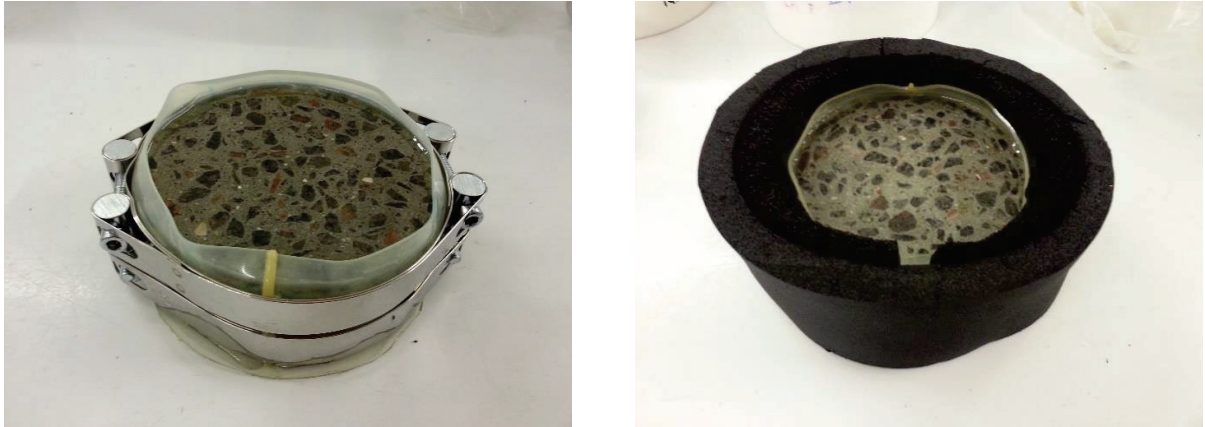
Figure 1: Specimen with hose clamps before (left) and after (right) all surfaces except the test surface had been covered with thermal insulation.
