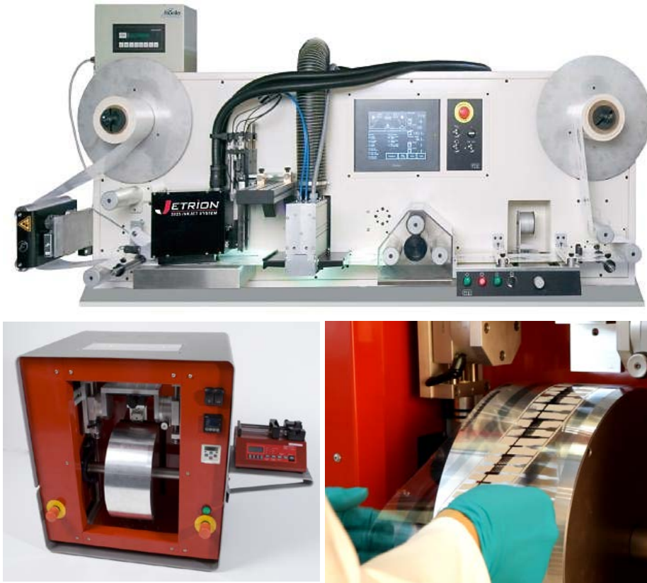
Figure 6.2: Bench-scaled machinery that mimics full-scale roll-to-roll processing: a roll-to-roll printer/coater from Grafisk Maskinfabrik (top) and a roll coater from FOM Technologies (bottom).
