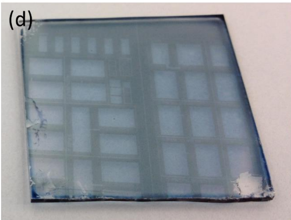
Figure 1. Patterning of VPP PEDOT:Tos. (a) The patterning procedure, (b) an example of a complex image patterned in the polymer, (c) electronic circuit patterned on Au substrate with minimum linewidth of 10 μm, line pattern on Au with (d) and without (e) the post polymerization baking step.
