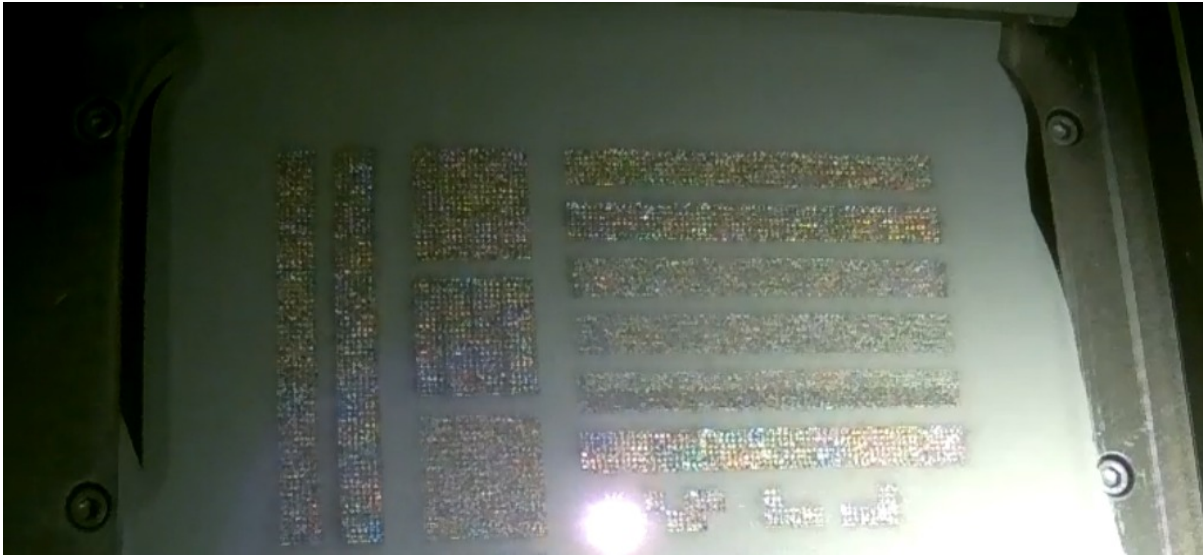
Figure 6 Manufacturing components by selective laser melting using optimized cellular scanning strategies
