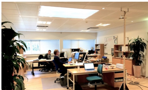
Fig. 1 Test office with mixing ventilation system
