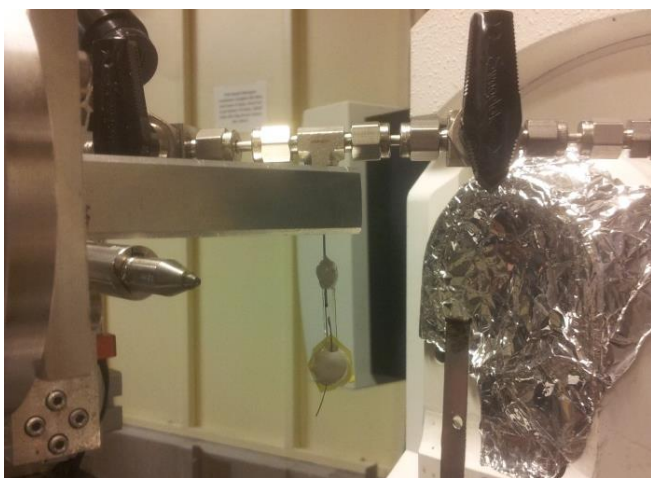
Figure S1: A picture of the capillary battery measured at the Maxlab II, beamline 711.
