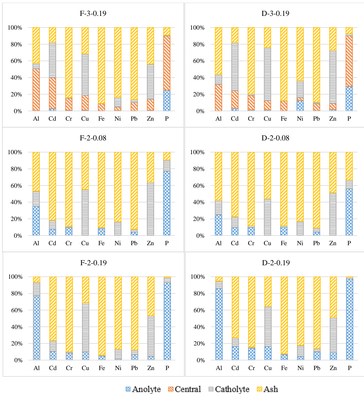
Figure 5. Percentage of heavy metals and phosphorus in the different matrices after the ED treatment in the 3C and 2c-cell design.
