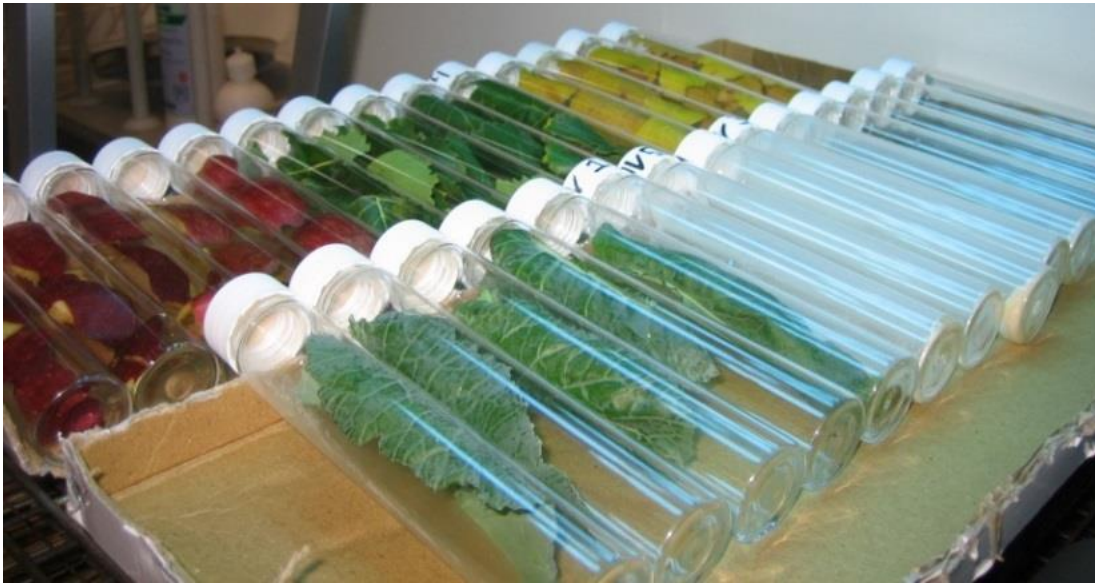
803 Figure A1. Plant leaves inserted in UV-B transparent vials. Note vials without leaves are used as blank 804 controls.
