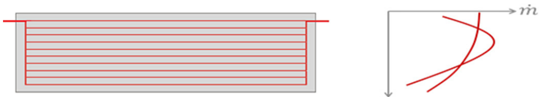
Fig. 2. Example flow distribution in a harp collector [11].
