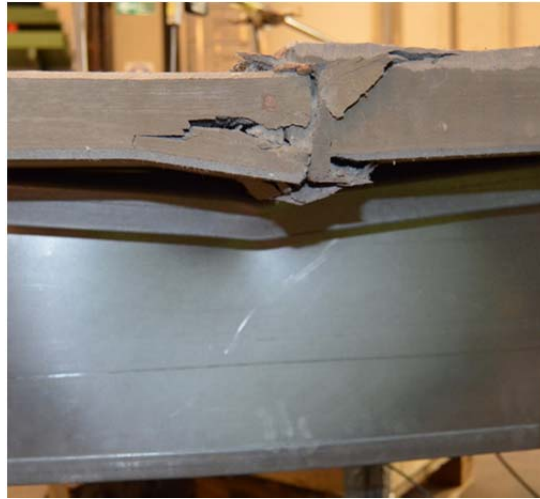
Figure 8.14 Compression failure of MP panel (second panel) at mid-span
