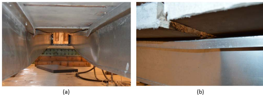
Figure 8.13 Failure of MP (first panel); (a) buckling of steel joists under one of the loading point and (b) subsequently failure of the connection between steel joists and the cast-in elements (first panel)
