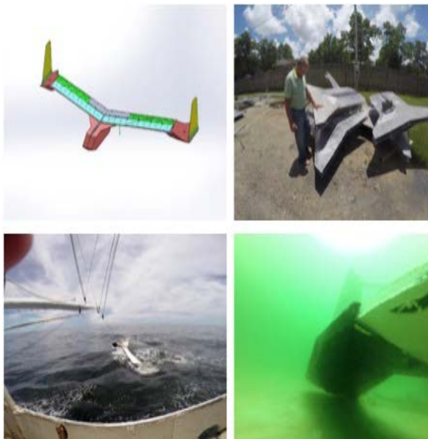
Figure 7.4.14. Wing Trawling System used for tropic shrimp trawling in the Gulf of Mexico ( images courtesy of Philip Walsh – Memorial University )
