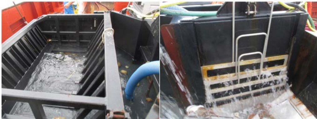
New deck hopper on-board GO31. Left: Stone catcher. Right: System to maintain and adjust water level in hopper.
