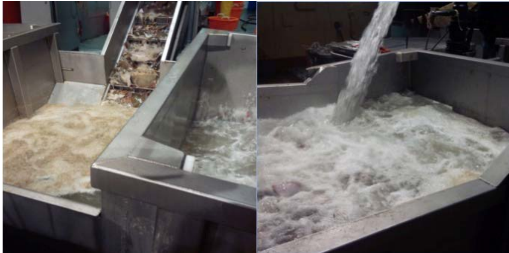
New deck hopper with water and air supply on-board SC25 (left). The water level in the hopper is controlled by using hydraulic slides (right).
