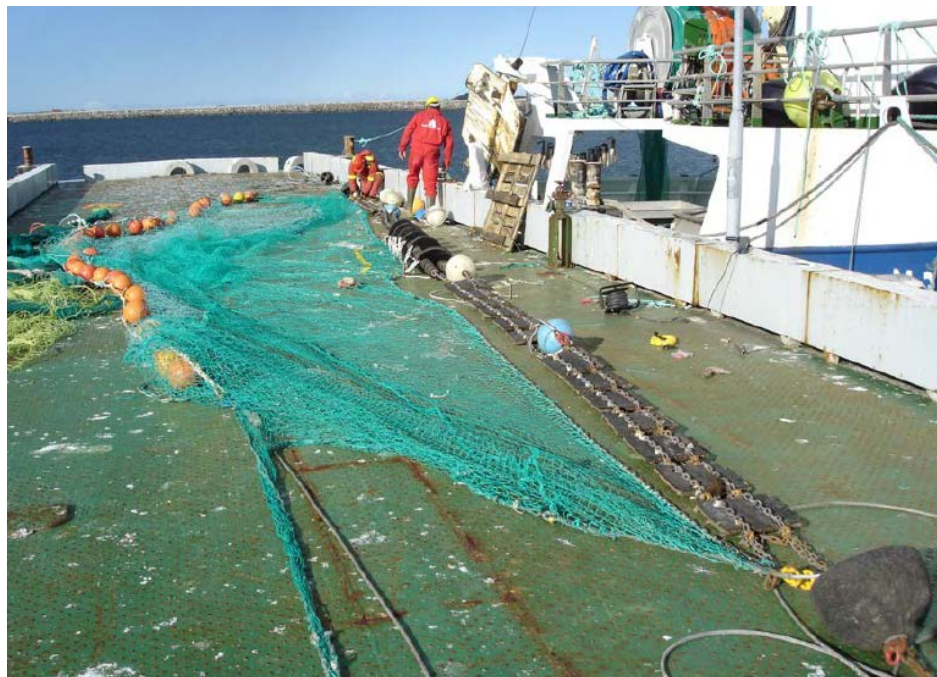
Figure 7.4.12. Self-spreading plat gear developed by Hansen and Valdemarsen (2006).
