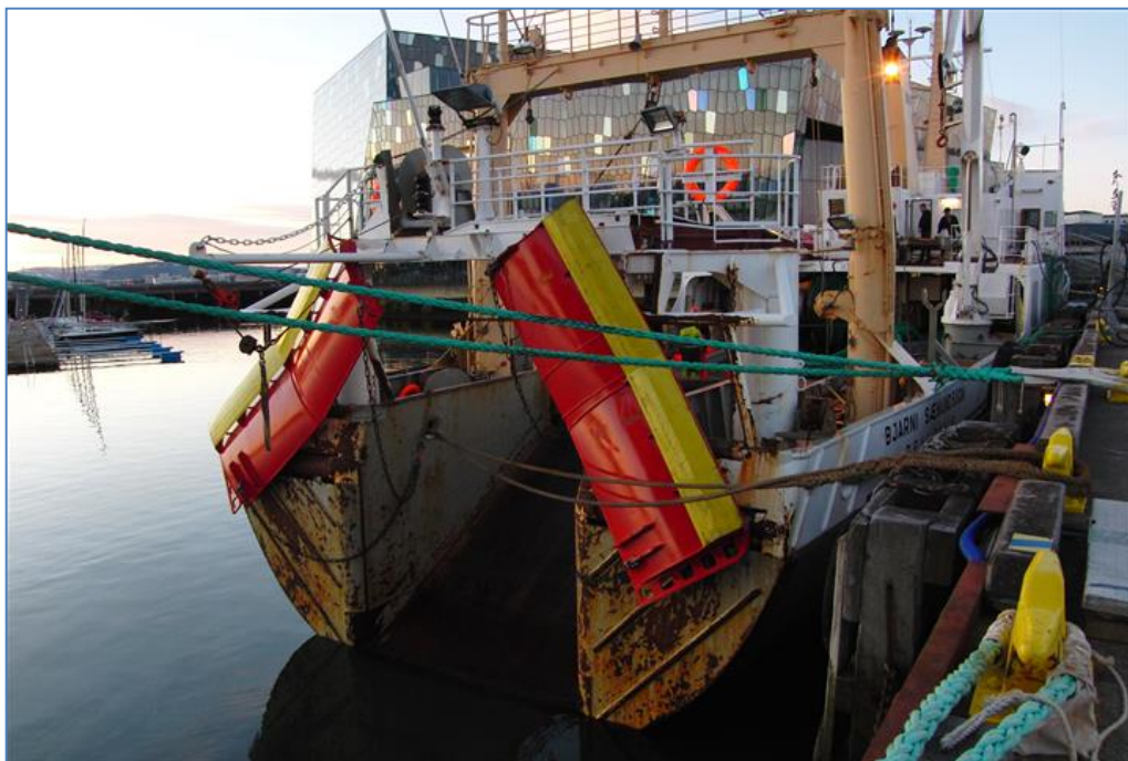
Figure 7.4.5. Ekkó trawl door developed by inventor Smári Jósafatsson in Iceland.
