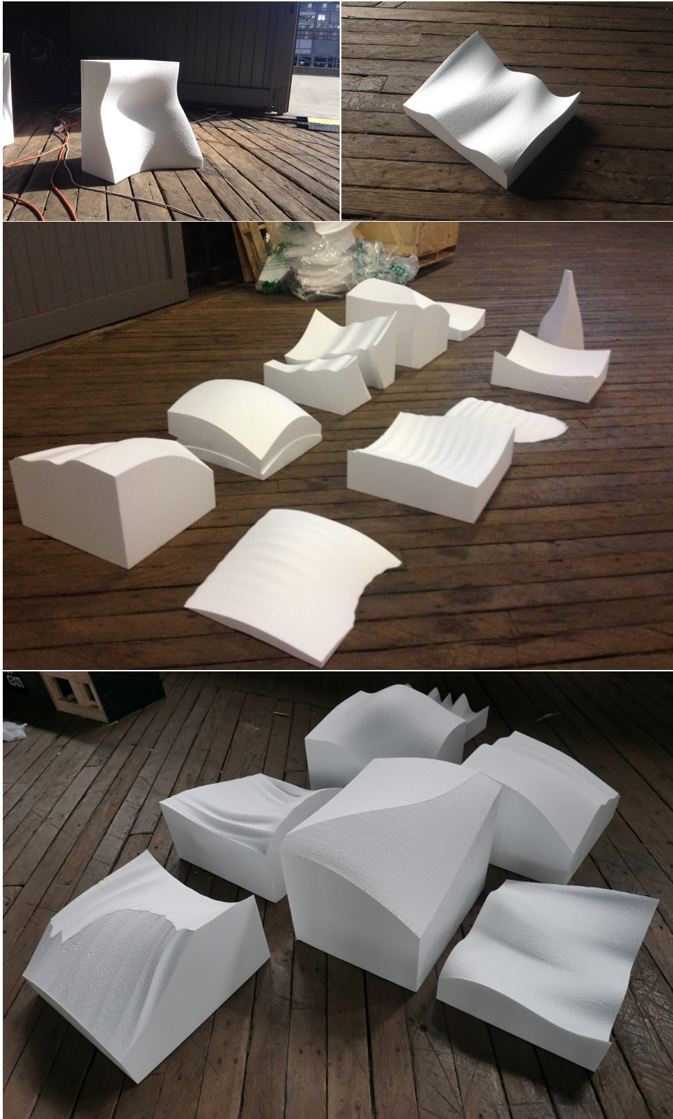
Figure 4.7: Single block designs cut at the RobArch 2016 Superform workshop. The bottom photo contains blocks that were cut twice.
