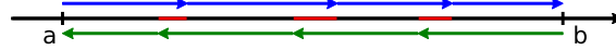
Figure 6.7: On the black axis, we have the parameter interval [a, b] for the sweep curve. The blue arrows show the segments that can be well approximated by elastica, based on the bisection method. The green arrows show the same but with the method used on the reversed curve, i.e. from b to a . The red regions are suggested for subdivision, since any segment from one red region to the next can be well approximated.
