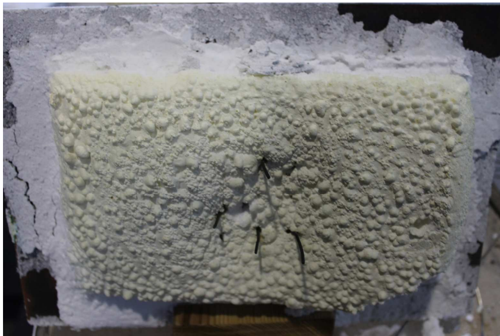
Figure 4. Photo of expanded char after 3 hours of heating in the furnace. The five uncovered metal thermocouples, placed above the char, can be seen close to the center of the char surface. The thermocouples already covered cannot be seen.
