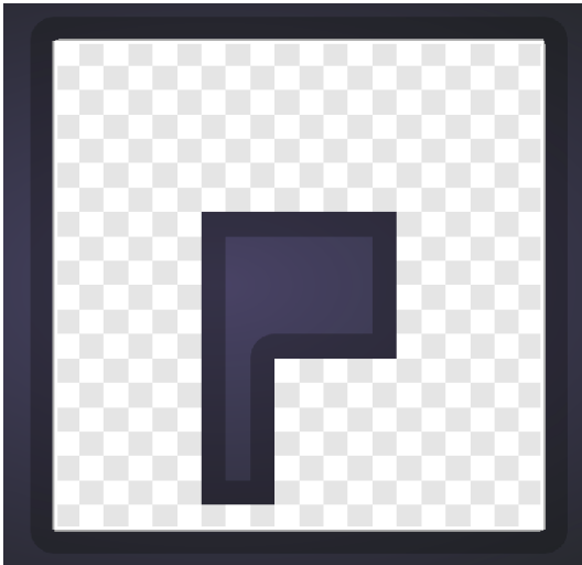
(a) Defining the design domain (size and excluded elements). The checkerboard shows the actual element size.
