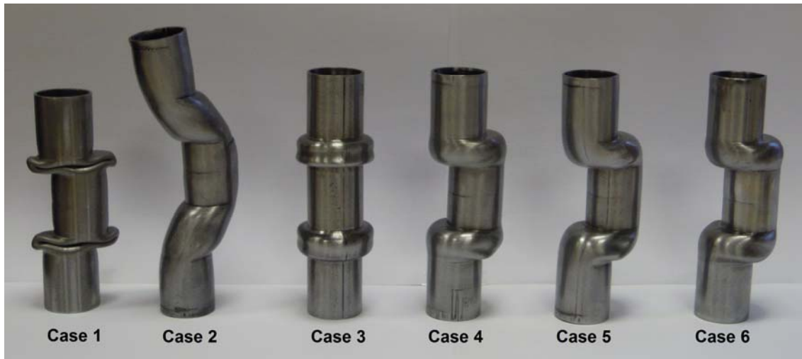
Figure 5 – Tubular components obtained from different movements of the vertical and horizontal actuators of the double-action tool system showing non-appropriate (Cases 1 to 3 of Table 1) and appropriate (Cases 4 to 6 of Table 1) modes of deformation.
