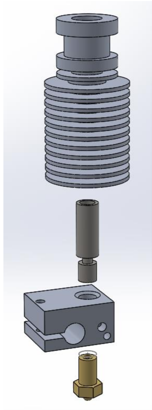
Figure 4 E3D HotEnd extruder; from top to bottom: heatsink, heatbreak, heater block, nozzle (modi_ed from a model from GrabCAD)
