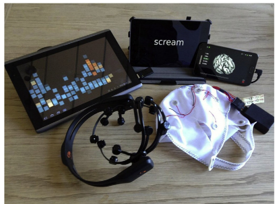
Fig. 3. SBS2 mobile neuroimaging apps for neurofeedback training, presentation of experimental stimuli, and real-time 3D source reconstruction, running on Android mobile devices via a wireless connection to an Emotiv or Easycap EEG setup.
