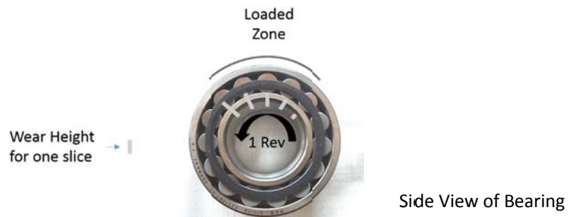
Figure 6. Diagram representing the accumulation of wear on the inner race from the contributions of each roller in one revolution. Wear accumulation is signified by the grey bars. (modified from (Wuxi Handa Bearing Co. Ltd 2016)) This figure shows that the wear on the inner race accumulates despite the varying loads it encounters as it passes the loaded zone.
