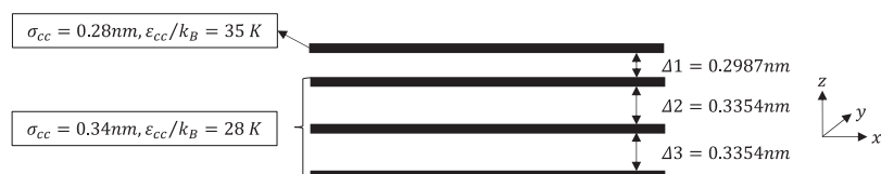
FIG. 1. Schematic illustration of solid arrangement of graphite. Top layer is modelled as a corrugated Crowell surface while the bottom layer is modelled as the Steele surface of infinite layers.
