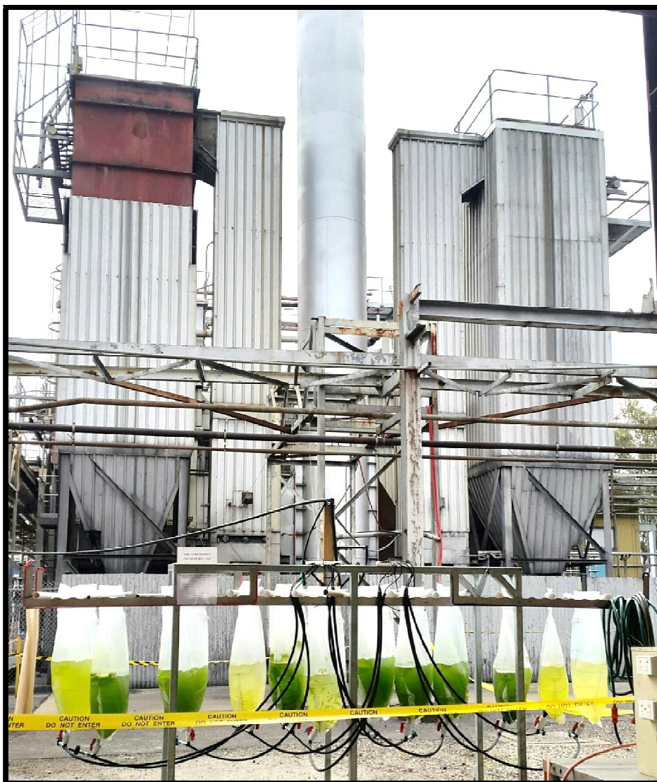
Figure 1. Experimental setup of photobioreactors connected to coal-fired flue gas.
