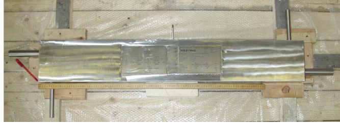
Figure 5: Printed Circuit Heat Exchanger (PCHEX) used by VanMeter [6]
