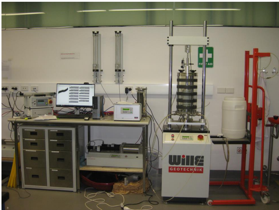
Figure 5-1 Triaxial testing system (Wille Geotechnik, 2013)
