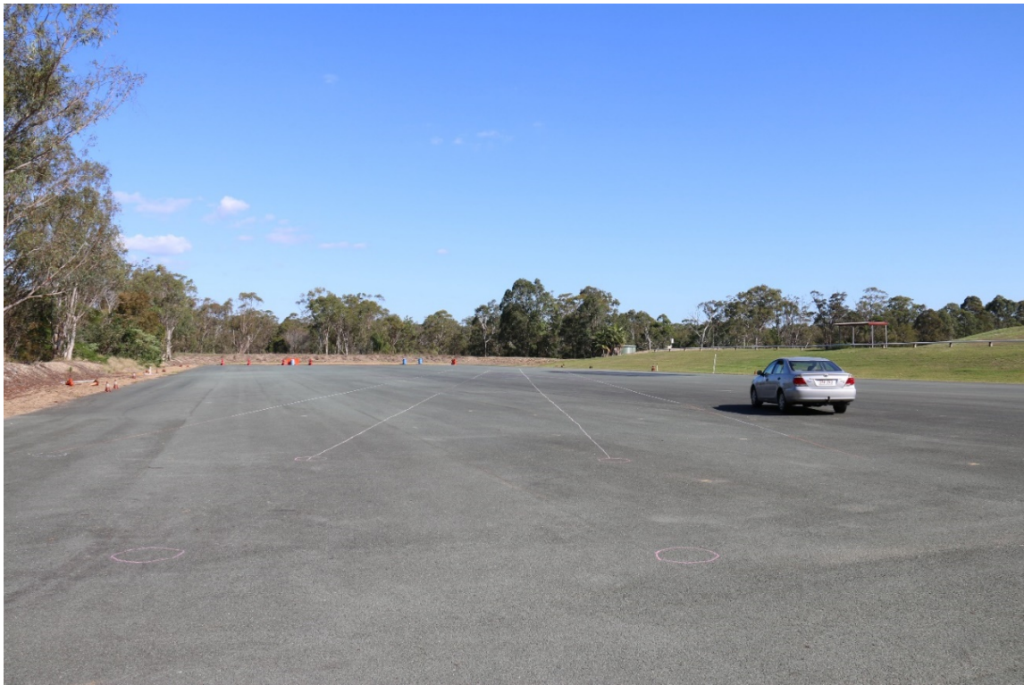
Figure 2d illustrates a typical view of the test site. Four lines were drawn to indicate three lanes. Participants drove in the central lane at the beginning of each trial and then changed to left or right lane. The lane marks appear a little faint in the photograph but were drawn with brightly coloured chalk and so were very easy to see at the test site.
