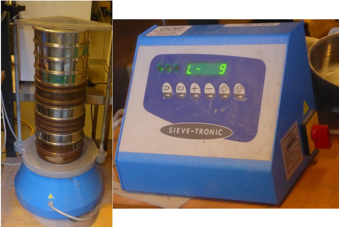
FIGURE 3: THE SIEVE SET AND MECHANICAL SHAKER AT THE UNIVERSITY OF QUEENSLAND LABORATORY.
