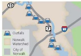
Locations of storm sewer outfalls in Norwalk River and Harbor.
