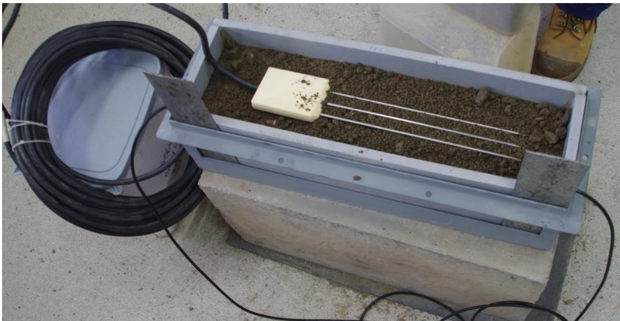
Figure 2: Positioning the TDR rod probe sensor within the UBG material sample.
