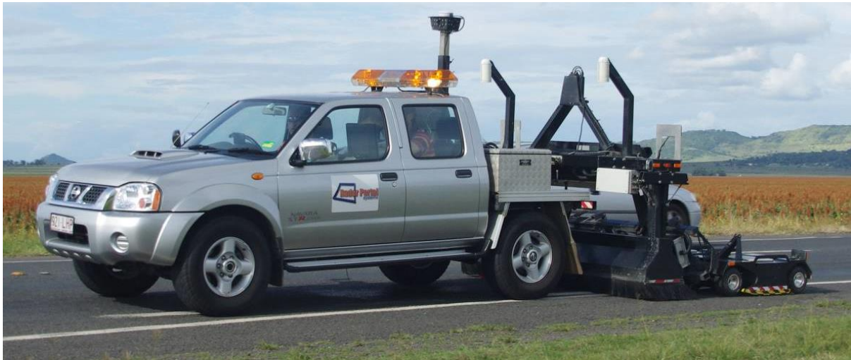
Figure 1. Roadscout 2 system incorporating a highway-speed 24 channel NM-GPR system and ground coupled antennas.
