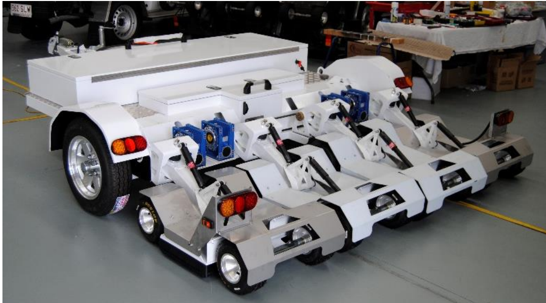
Fig. 1. Updated 3D NM-GPR system.
