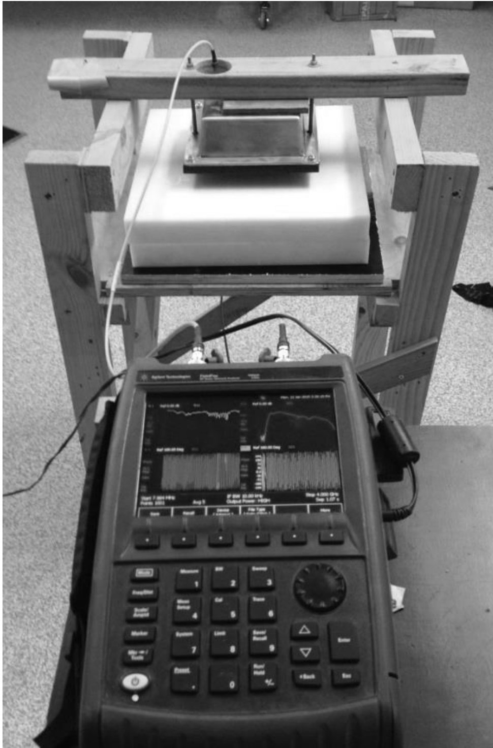
Fig. 4: VNA measurements with fixed antenna separation through samples of nylon and a ply sheet.
