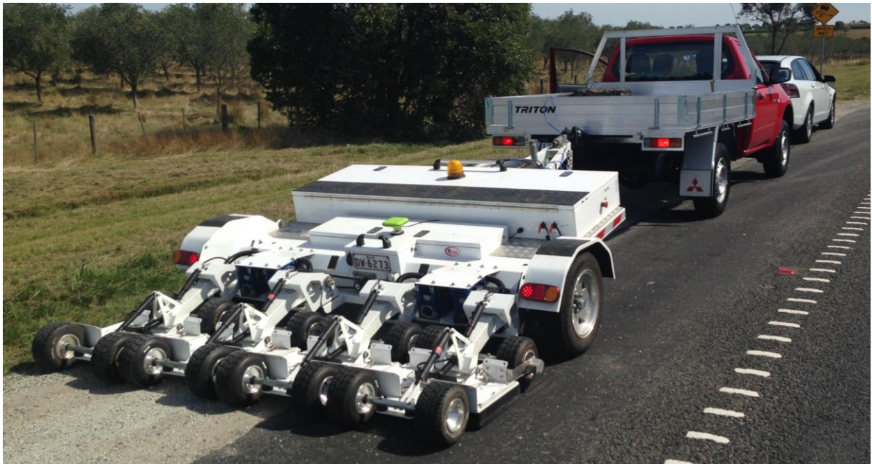
Figure 2-4: Second generation NM-GPR system incorporating a traffic-speed 3D ground-coupled antenna array
