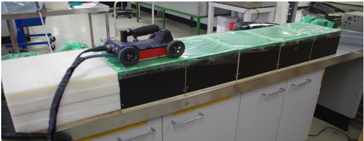
Figure 3: Collecting impulse GPR measurements of nylon and moisture-varying UBG samples M1 to M5.
