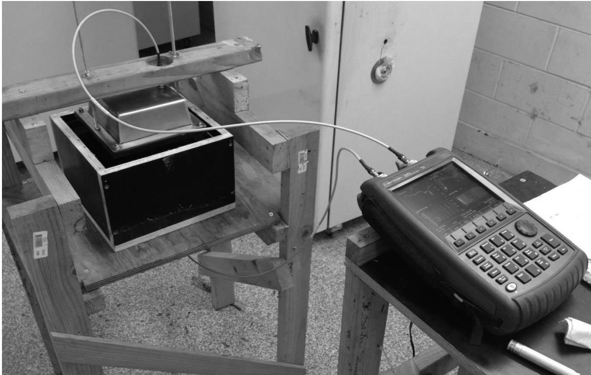
Fig. 7: MFS test configuration used for measuring a 170 mm deep sample of distilled water shown prior to complete filling of the sample box.
