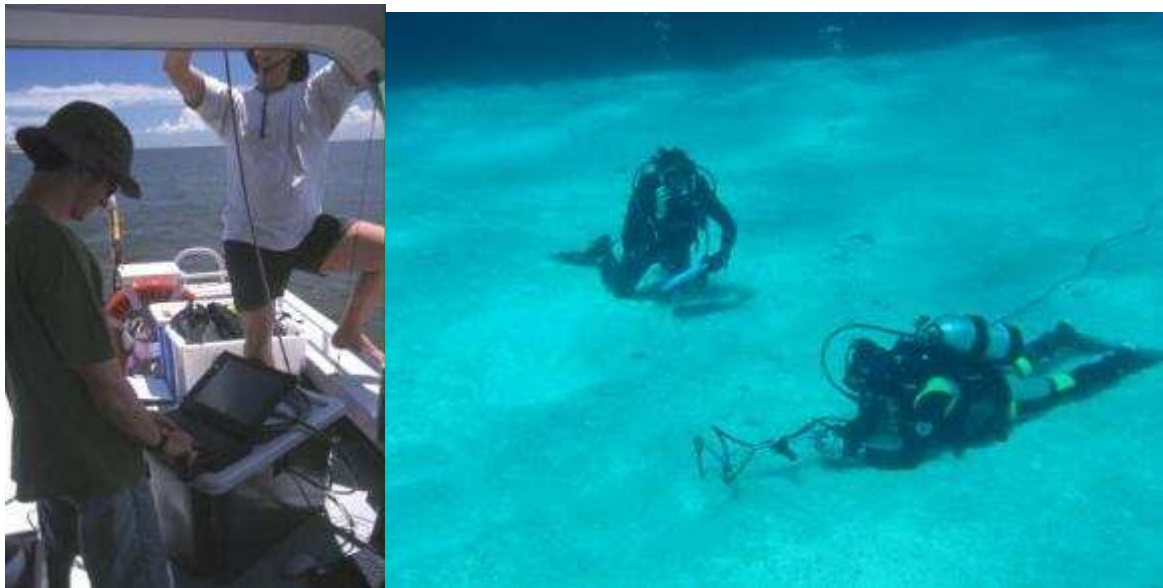
Figure 7: Example of underwater spectral measurement using a HydroRad-4 spectroradiometer operated at the surface (left) while a long optical cable with up- and down welling sensor head is positioned by a diver above the target material(right). Through underwater communication devices the diver communicates with the spectrometer operator to inform each other about the status and the type of measurement..
