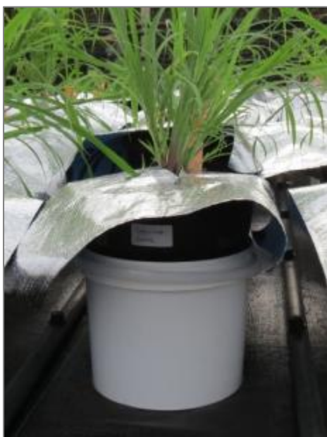
Figure A2.2. Image showing the double-pot system used for treatments in which plants were growing into saline soil. Saline water was used to flush the soil contained in the black pot. The leachate collected into the second pot (white bucket) was used to monitor the soil liquid phase electrical conductivity (e.g. salinity).
