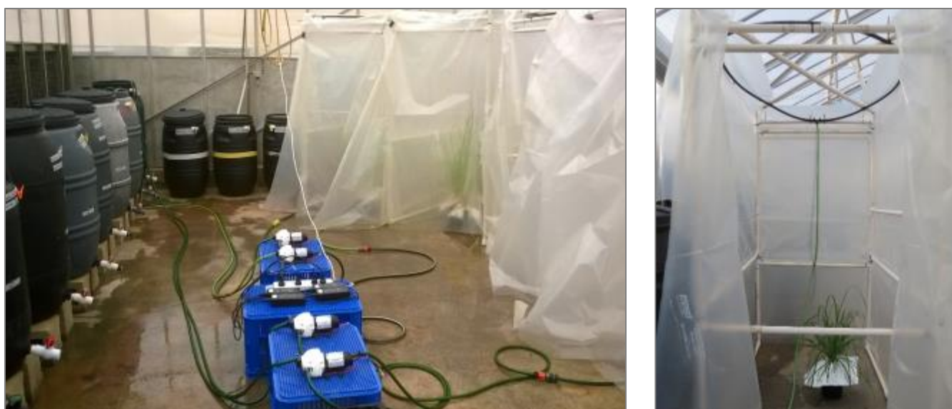
Figure A2.3. Images of the overhead irrigation system. On the left, the system set-up; plants were irrigated in chambers (right) connected to water pumps (middle) and 200L drums (left) containing relevant treatments. On the right, details of an irrigation chamber; water piping equipped with Netafim microjet nozzles was fitted above the structure to enhance plant foliage wetting.
