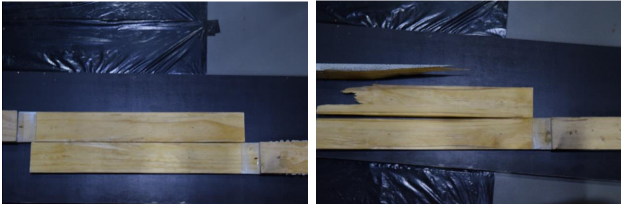
4 5 Figure 50: 150°C temperature test failures. Test 1 (left). Test 2 (right)
