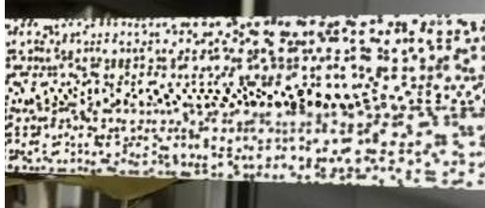
5 Figure 44: Speckle pattern distribution over the single-lap bonded joint.
