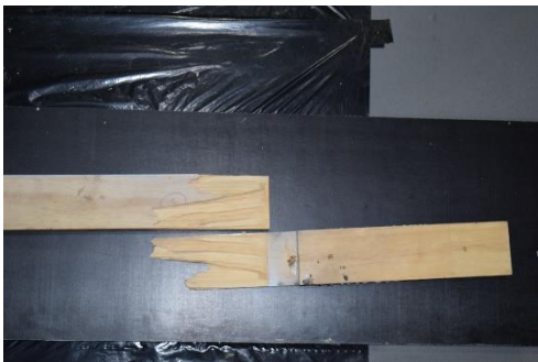
13 Figure 49: 80°C and 110°C temperature test failures. 80°C Test 2, 80°C Test 3, 80°C Test 5, 14 110°C Test 2, 110°C Test 3 (clockwise from top left)
