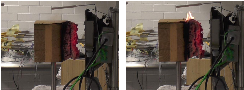
8 9 Figure 27: Bond line separation and re-ignition near the top surface of a sample exposed to 55 10 kW/m 2 heat flux.
