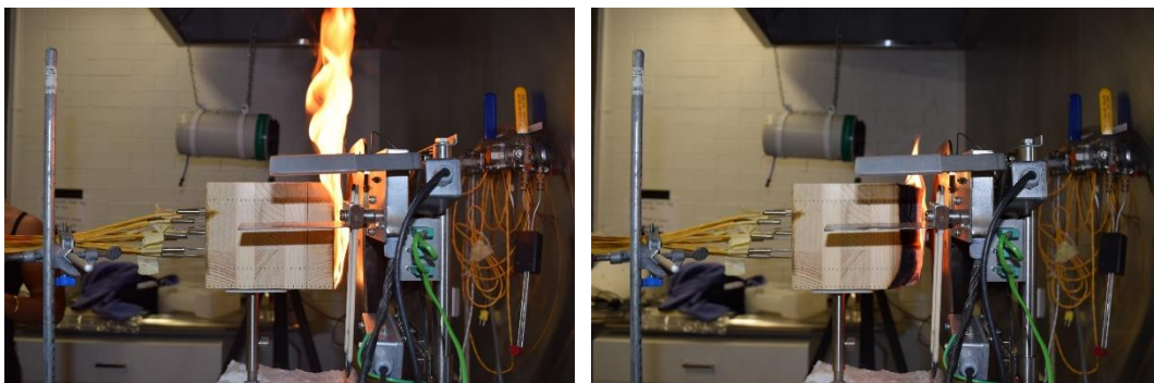
Figure 11: Flame height during early stages of transient burning (left) and steady-state (right)
