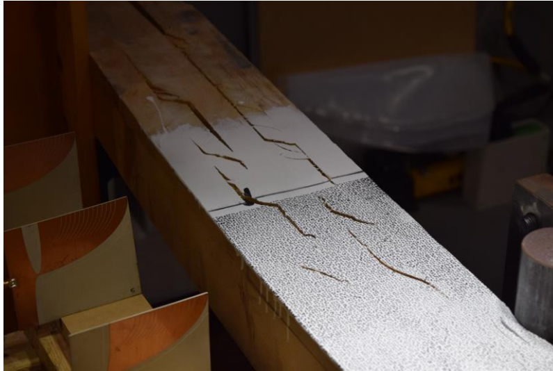
4 5 Figure 63: Rolling shear and debonding in the second and fourth plies of a CLT beam in Test 6 3 at ambient temperature 7
