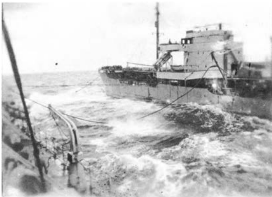
HMS "Havelock" (left) oiling from tanker in mid-Atlantic, while maintaining convoy speed.
