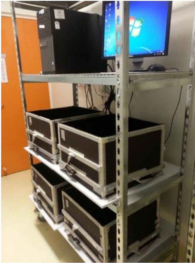
Figure 2-3 Locomotor activity boxes equipped with infrared beam detectors and the controlling computer
