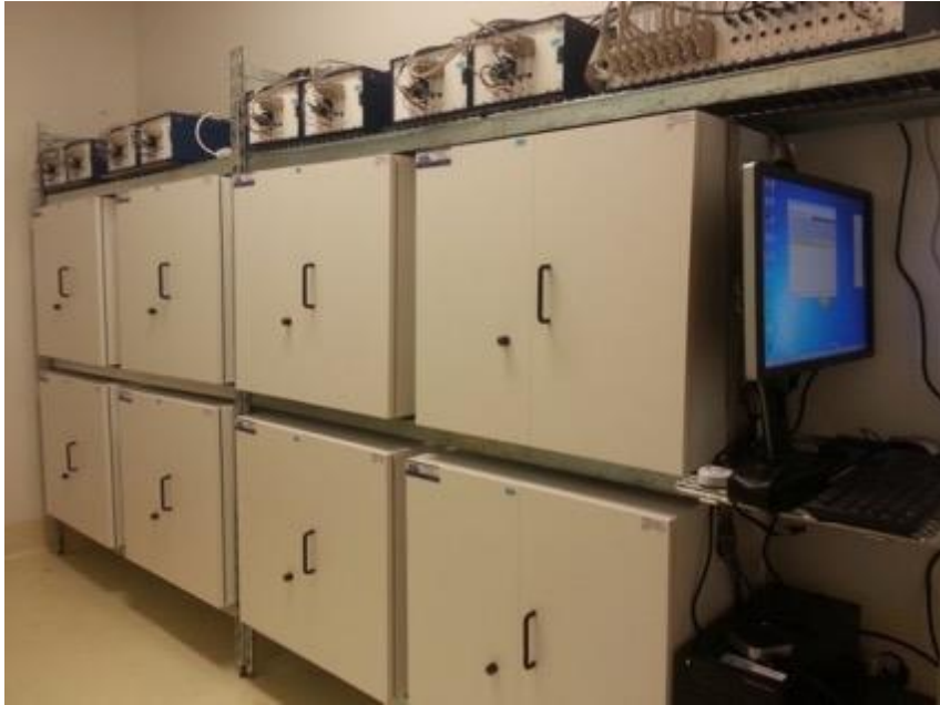
Figure 2-1 CAR chambers used in my study (a) Eight sound-attenuating chambers, aversive stimulus generators and the controlling computer were shown. (b) A two-way shuttle box inside a sound-attenuating chamber was shown.
