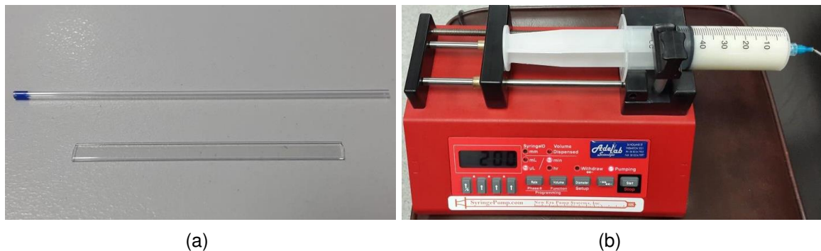
FIGURE 3.16: (a) Circular and rectangular capillary tubes used to model blood vessels and (b) syringe pump to push liquid (blood phantom) through these channels.
