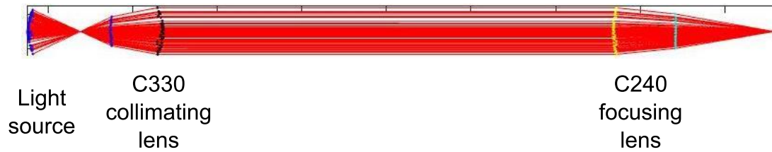
FIGURE 3.2: Numerical optical system including Thorlabs, Inc., C330TME-B and C240TME-B model lenses.
