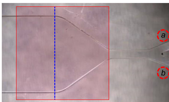
FIGURE 5.2: Two inlet rhombic microfluidic channel. Flow is pushed through from inlet a when a stop valve is placed on b . Red shaded square shows the scan area and signal to background ratio is calculated along the blue broken line.
