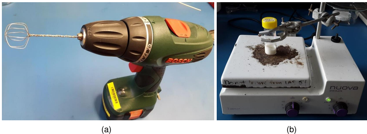
FIGURE 3.14: (a) Drill and whisk as mechanical stirrer and (b) magnetic stirrer hotplate and a container containing a magnetic bar in it.
