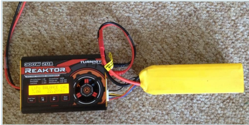
Figure 28: Balance charging a single LiPo 5S battery
