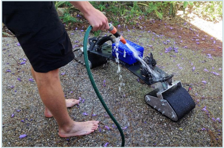
Figure 25: Spraying the board with water
