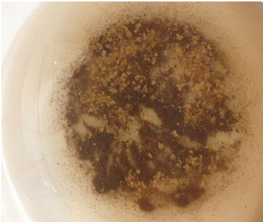
2016/08/05 - Separator 2. Condenser water, operating.
