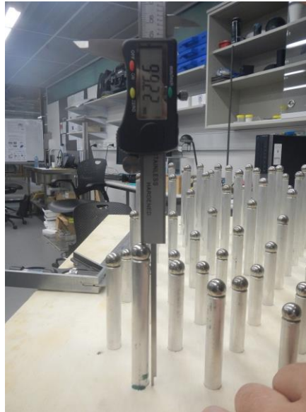
Figure 29 – Method used to estimate tolerance associated with automated mould setting
