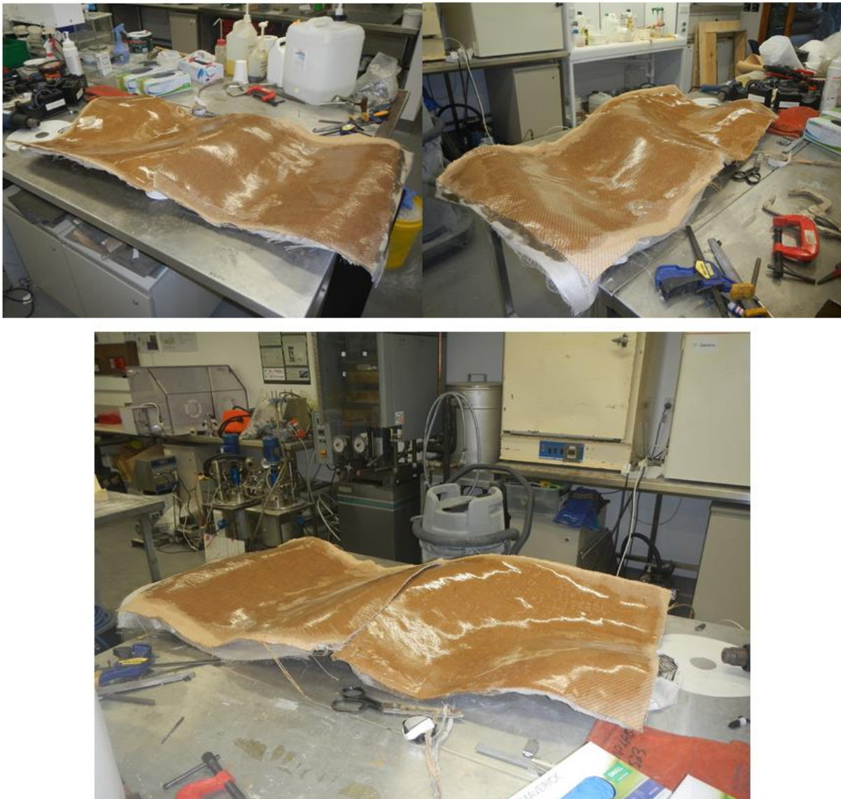
Figure 35 – Assembly of two sample panels.
