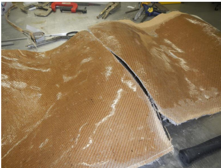
Figure 36 – Defect between panels.
