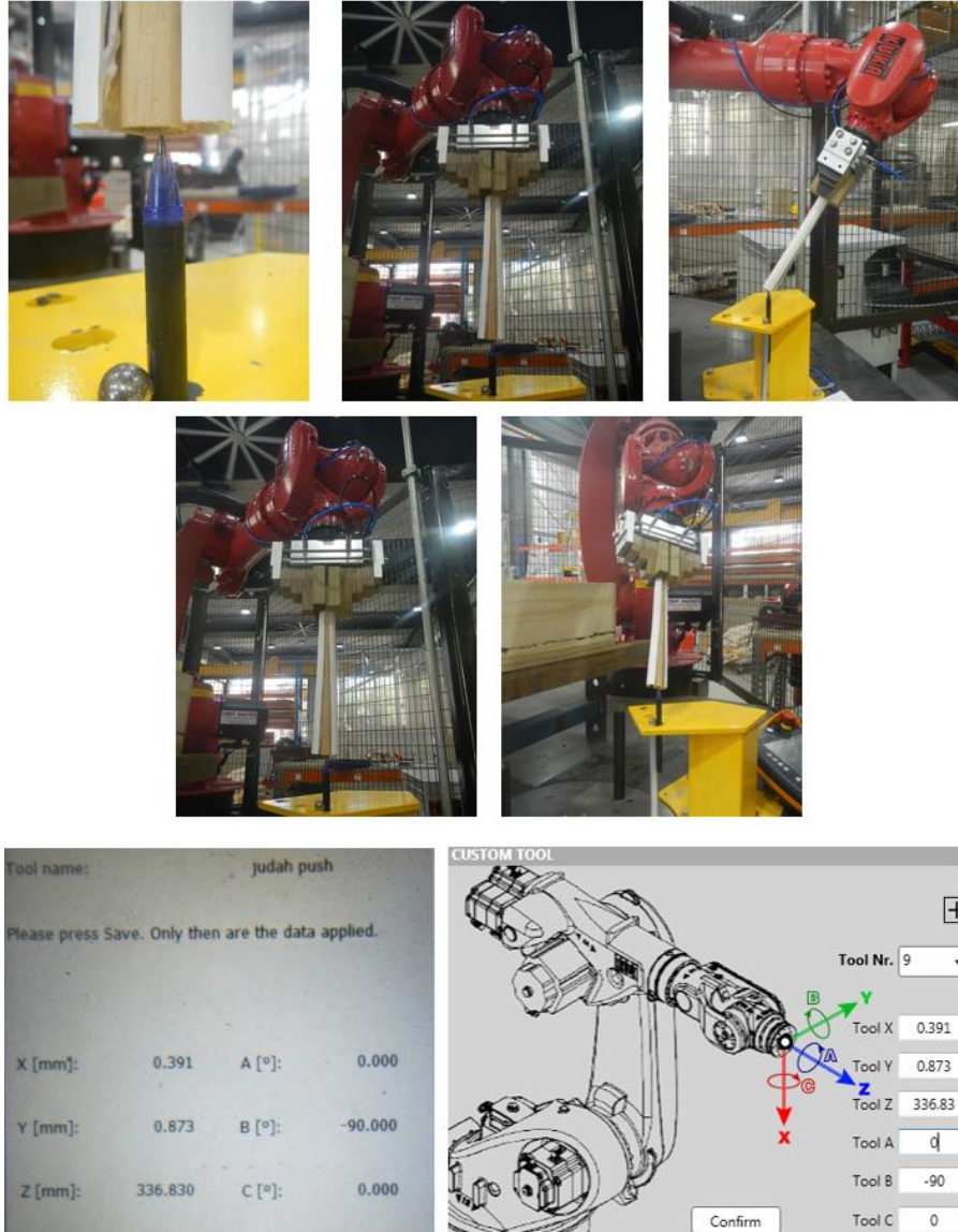
Figure 23 – Process for tool calibration in order from left to right and descending
