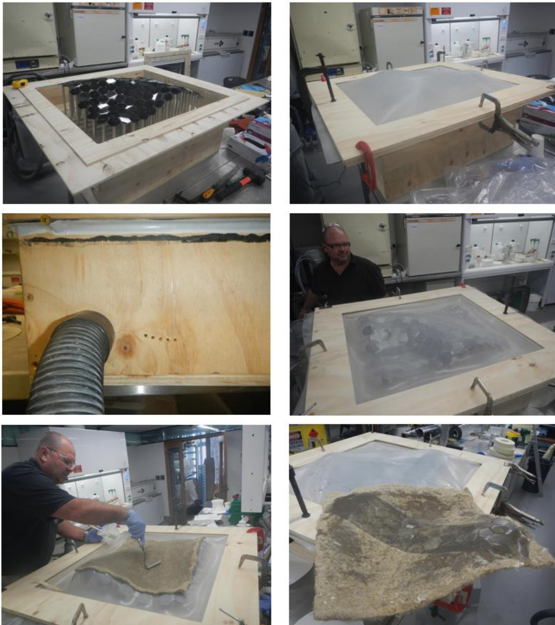
Figure 31 – Process for panel fabrication in order from left to right and descending.
