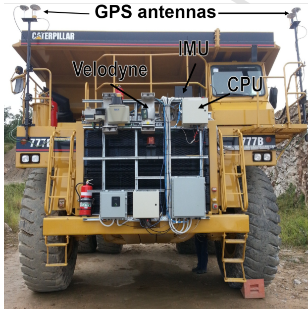
Figure 3: Mounting of Velodyne, and pose solution hardware on a Caterpillar 777B haul truck.
